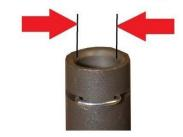
The earlier design has a smaller pipe fitting.
